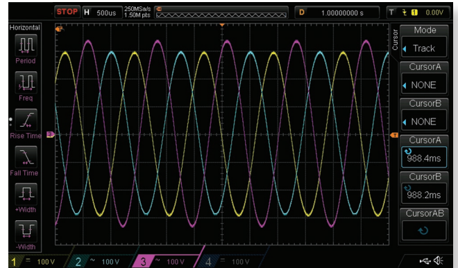
Three Phase Unbalance Voltage Test Captured
