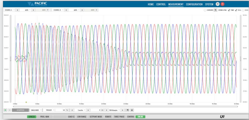
Waveform Example of Inductive Motor Emulation: 400Hz, 55A (AGX Series overload from 42A)
